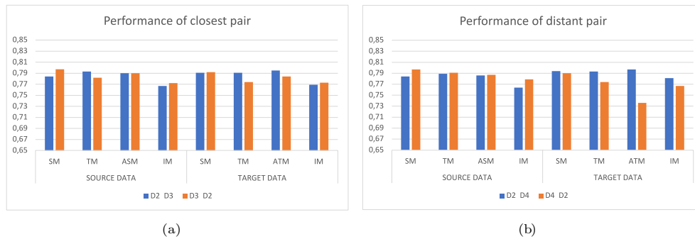
Fig. 5 Experiment A2-DIBCA++: Performance comparison of the closet and distinct pairs of devices based on the similarity of the data sets. The notation Dx-Dy represents that Dx is the source and Dy is the target. Each plot presents the performance (using
