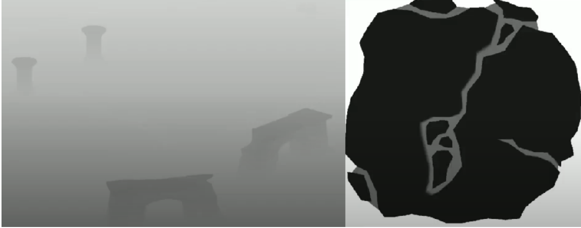
Figure 3.1: Two pictures, the left is a texture generated by Shadow Mapping. To the right is a GINT generated with the same shader setup. This is the first GINT created, although it was used for collision detection rather than path planning, a different purpose to the implementation of GINT in this thesis makes use of.
