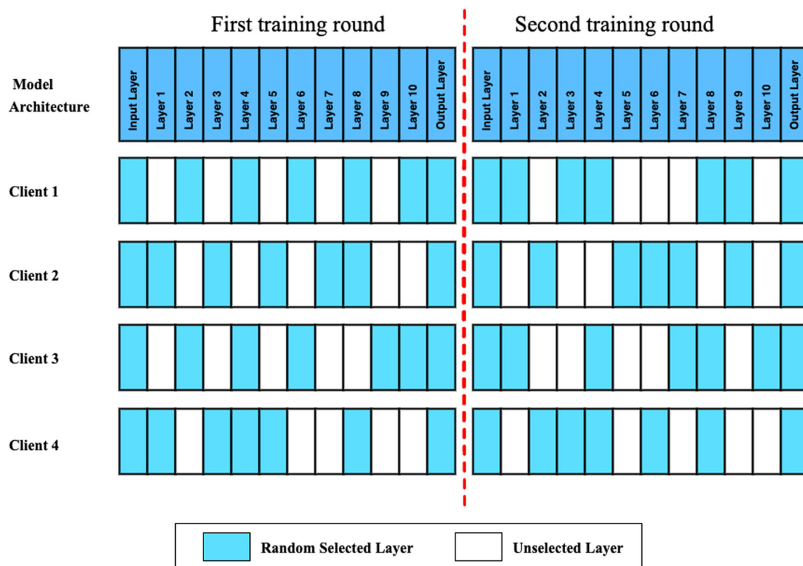
Fig. 1 The abstract diagram depicts the proposed approach for training the ML model with four clients in the FL context. Where each client independently selects 50% of the entire model layers randomly during every training round
