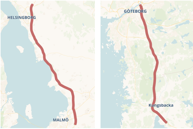
(a) European road E6 between Malmö and Helsingborg. The freeway is 64 km long, has 59 links with a free-flow travel time of 34.2 minutes. The posted speed limit is 110 km/h for all links. (b) European road E6 between Gothenburg and Kungsbacka. The freeway is 35.7 km long, has 49 links with a free-flow travel time of 24.5 minutes. The posted limit varies between 70 and 110 km/h.
