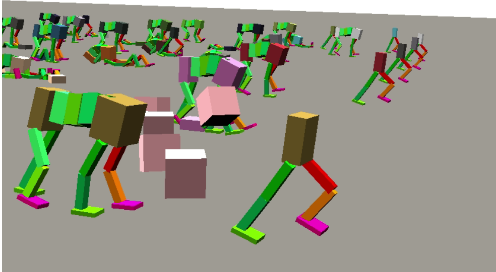
Figure 1.5: Screenshot of the application developed for the thesis. It shows walking bipeds and quadrupeds, simulated using the implemented pose-driven feedback locomotion algorithm. In this screenshot an example of interactivity is shown by having boxes thrown at the characters to disrupt their balance.
