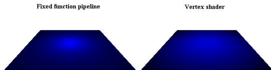
Figure 9. Pointlight with the fixed function pipeline versus a vertex shader
