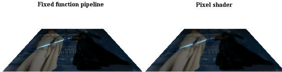
Figure 12. Multitexture blending with the fixed function pipeline versus a pixel shader
