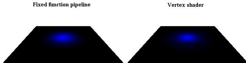
Figure 10. Spotlight with the fixed function pipeline versus a vertex shader
